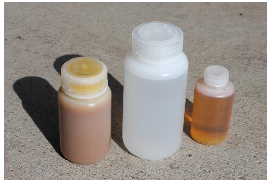
Photo 1 The Colours of the Samples from right to left; Reclaimer Feed, Reclaimer Product, and Process Fluid.
